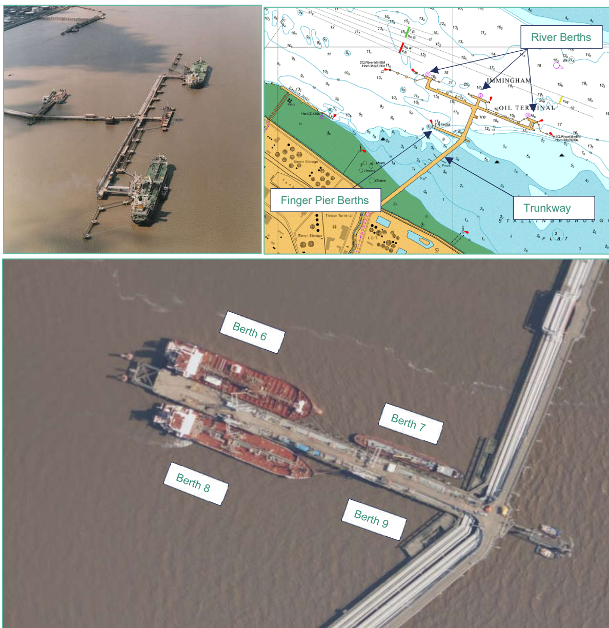
Figure 4: Top left aerial view of IOT berths (source: humber.com), Top right: Nautical chart showing Trunkway, finger pier and river berths, and Bottom: close up aerial view showing the finger pier (showing berths 8 and 6 occupied by coastal tankers and berth 7 occupied by a bunker barge), Trunkway (pipe tracks are white/light grey) and small workboat berth opposite the finger pier.
